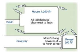
2. **Disconnect your downspout.** Measure your downspout from the top of the standpipe and mark it at 9 inches above the standpipe. Depending on the length of your extension, you may need to cut it higher. Cut the downspout with a hacksaw at the mark, and remove the piece. Cap or plug the standpipe with either a wing-nut test plug or rubber cap with hose clamp. Do not use concrete to seal your standpipe.
